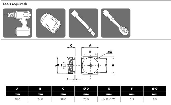
**NOTE** Screws for the anti-vibration mounts to the wall are not provided, they should be suitable for the weight and surface that the drive will be mounted to. See Drive user guide for weights and dimensions.
